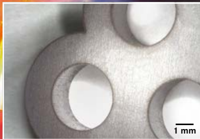
Precision cuts in up to 4-mm-thick metal sheets (4-mm-stainless steel) – low taper/sharp edges
