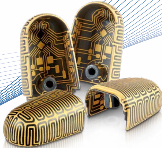
Finger tips for a robot hand (Source: Citec, Bielefeld University)
