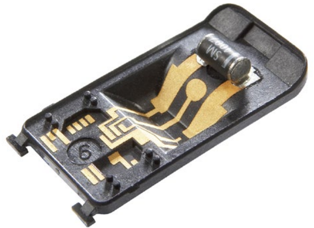
Figure 6a and 6b: The structure may be connected via bonding or can be assembled with electronic components.
