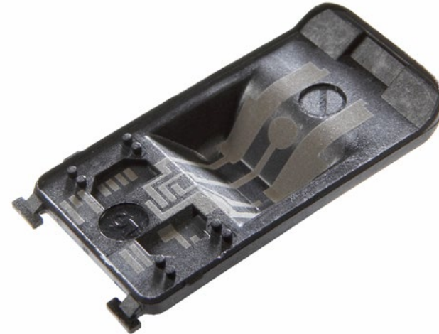
Figure 4a and 4b: The laser beam has structured the blank and has activated the additive.
