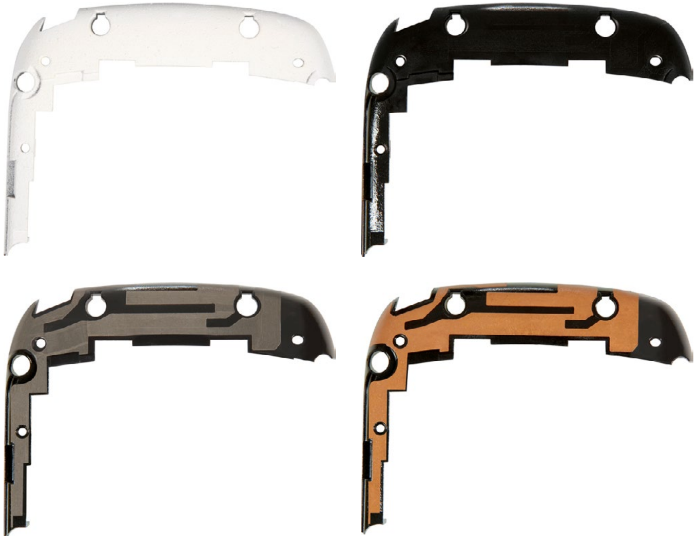
Figure 9: After building up a body in rapid prototyping it is painted with ProtoPaint LDS. The laser transmits the projected circuit structures and metal layers are built up using an electroless bath.
