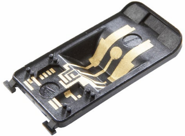
Figure 5a and 5b: In a currentless metallization bath copper settles on the structured parts.
